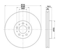
HELLA 355128191 Front Brake Disc Volvo XC90 (Externally Vented)
